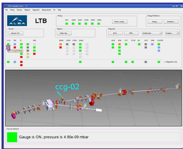
Figure 3: Main Graphical User Interface for the Linac to booster transfer line.
